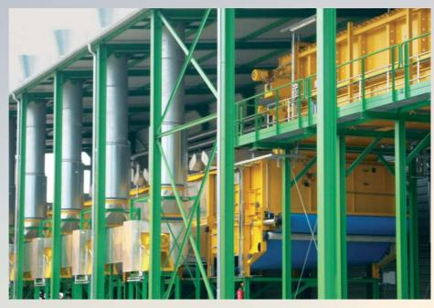
The fabric belt drier in a wood pelleting plant
